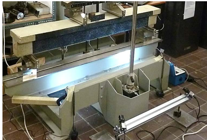
Figure 2 - Full beam test set-up with DIC cameras
