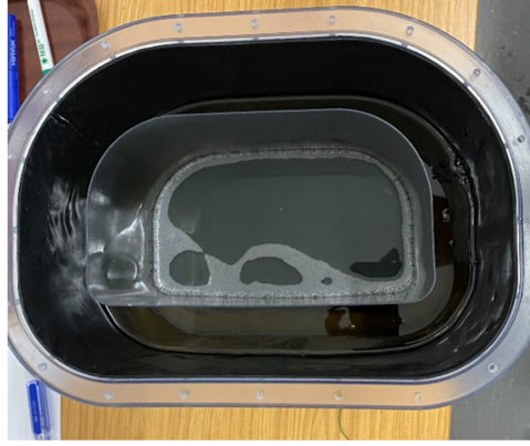
Figure 3.12: Top view of filled multi-layered SPEAG chest phantom.
