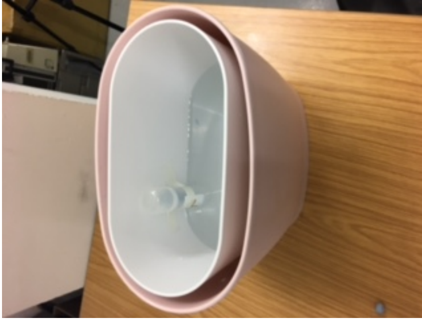
Figure 3.6: The lung COVID-19 infection fabricated phantom.
