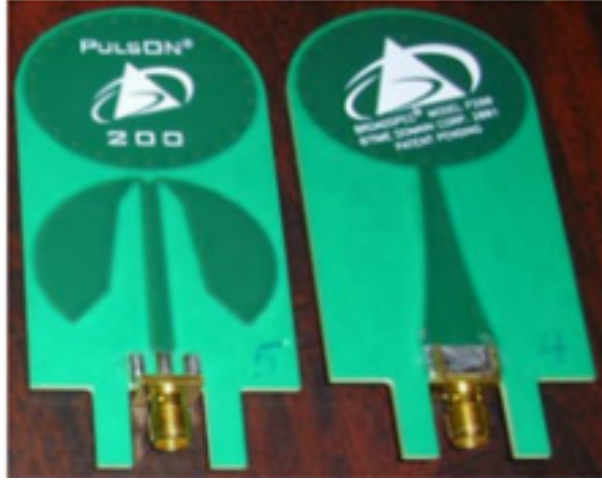
Figure 3.1: The PulsON P200 UWB Antenna [38].
