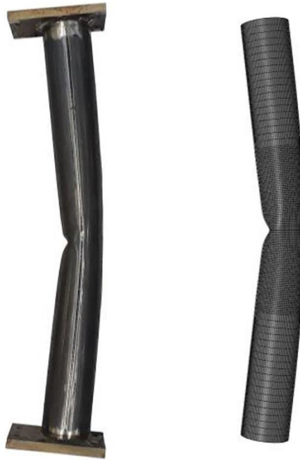
Fig. 3: Typical failure modes obtained experimentally and numerically [22].
