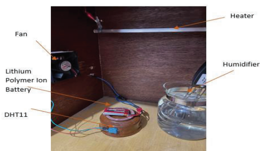
Figure 2. The experimental test area in the Temperature/Humidity chamber.
