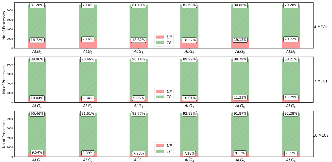
Figure 31 Comparison Of The Ratio Of Processes That Missed Their Deadline To The Processes That Failed To Meet Deadline. TP (Timely Process) Is Used To Denote Processes That Meet Execution Deadline While UP (Untimely Process) Is Used To Denote Tasks Processes that missed deadline for Exp_2
