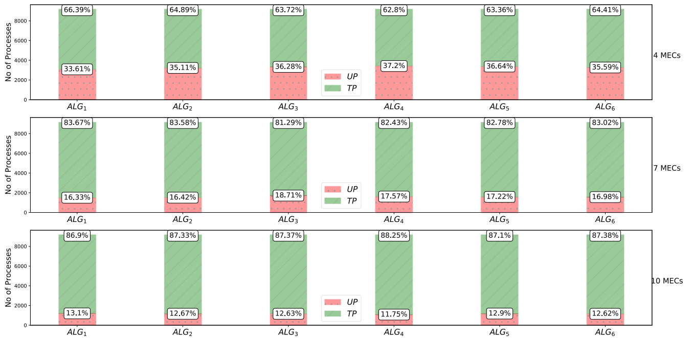
Figure 26 Comparison of The Ratio Of Processes That Missed Their Deadline To The Processes That Failed To Meet Deadline. TP (Timely Process) Is Used To Denote Processes That Meet Execution Deadline While UP (Untimely Process) Is Used To Denote Tasks Processes that missed deadline for Exp1
