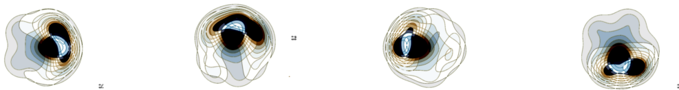
FIGURE 6.60: A combination of 5 transmitting position triplets for inclusion at 0^\circ , 90^\circ , 180^\circ and 270^\circ . SSIM images obtained using measured data with MWI device after performing artefact removal through local average subtraction artefact removal method at frequency 1 to 1.5 GHz.
