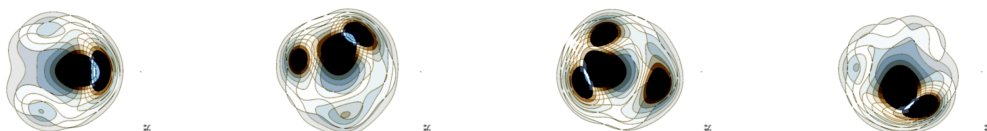
FIGURE 6.62: A combination of 5 transmitting position triplets for inclusion at 0^\circ , 90^\circ , 180^\circ and 270^\circ . SSIM images obtained using measured data with MWI device after performing artefact removal through summed symmetric differential artefact removal method at frequency 1 to 1.5 GHz.
