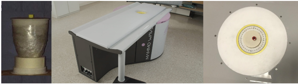
FIGURE 4.8: The fabricated head phantom is comprised of three different layers emulating the skull (bone), human brain, and the brain haemorrhage for using in MWI device.
