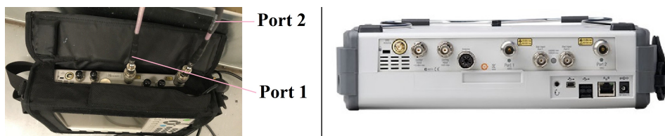
FIGURE 4.13: The VNA used in anechoic chamber. Port 1 is connected to the transmitting antenna and port 2 is connected to the receiving antenna.
