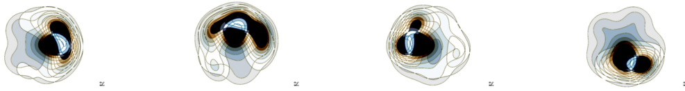
FIGURE 6.59: A combination of 5 transmitting position triplets for inclusion at 0^\circ , 90^\circ , 180^\circ and 270^\circ . SSIM images obtained using measured data with MWI device after performing artefact removal through rotation subtraction artefact removal method at frequency 1 to 1.5 GHz.
