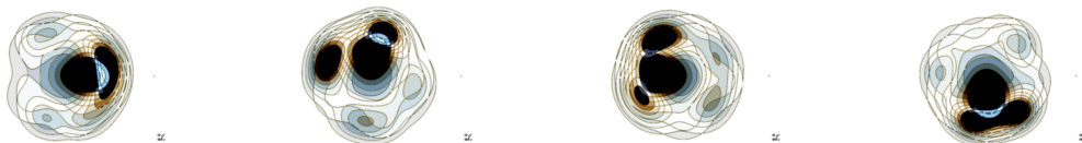
FIGURE 6.61: A combination of 5 transmitting position triplets for inclusion at 0^\circ , 90^\circ , 180^\circ and 270^\circ . SSIM images obtained using measured data with MWI device after performing artefact removal through differential symmetric receiver type artefact removal method at frequency 1 to 1.5 GHz.
