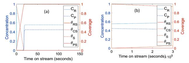
**Figure 4.** Estimated reactant and product concentration profiles (**left axis**) and surface species coverages (**right axis**) with respect to time for mechanism III at different scales of time on stream: a) Short times on stream up to 150 s. b) Large times on stream.
