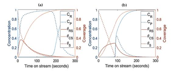
**Figure 6.** Estimated reactant and product concentration profiles (**left axis**) and surface species coverages (**right axis**) with respect to time: sensitivity analysis for Mechanism II, (**a**) with increased  $k_2$  by 100% and (**b**) decreased  $k_{-2}$  by 10% (**b**)  $\tau = 5$  s.
