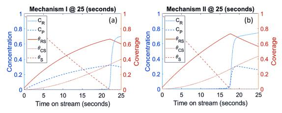
**Figure 3.** Estimated reactant and product concentration profiles (**left axis**) and surface species coverages (**right axis**) with respect to time: comparison between mechanism I (Fig. 3a) and and mechanism II (Fig. 3b).
