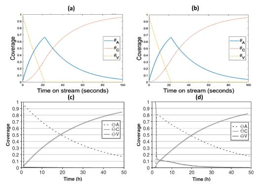
**Figure 10.** Estimated surface compound coverages: Comparison between CSTR (present study) and PFR (literature study), (a) mechanism I (elementary model, CSTR), (b) mechanism I (reduced  $k_1$  by 20% and increased  $k_{-1}$  by 10%, CSTR), (c) literature (elementary model, PFR), (d) literature (reduced  $k_1$  by 20% and increased  $k_{-1}$  by 10%, PFR.
