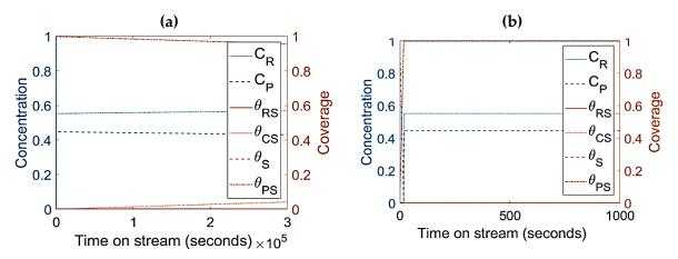
**Figure 8.** Estimated reactant and product concentration profiles (**left axis**) and surface species coverages (**right axis**) with respect to time: sensitivity analysis for Mechanism IV, (**a**) elementary model, using parameters values in Tables I and II (**b**) with decreased  $k_{-C}$  by  $10^{-5}$  and  $k_{C}$  unchanged.
