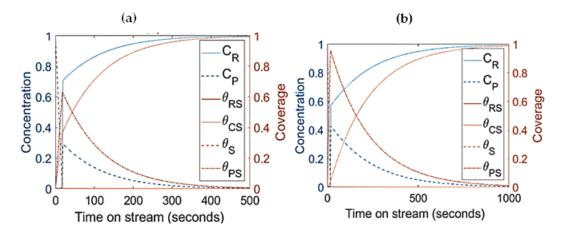
**Figure 7.** Estimated reactant and product concentration profiles (**left axis**) and surface species coverages (**right axis**) with respect to time: sensitivity analysis for Mechanism III, (**a**) with increased  $k_C$  by  $10^{-5}$  and  $k_{C2}$  unchanged (**b**) with increased  $k_{C2}$  by  $10^{-5}$  and  $k_C$  unchanged.
