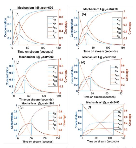
**Figure 9.** Estimated reactant and product concentration profiles (**left axis**) and surface species coverages (**right axis**) with respect to time: showing the effect of increasing catalyst amount. a:  $\rho_{cat}$ =600 g cm<sup>-3</sup>. b:  $\rho_{cat}$ =750 g cm<sup>-3</sup>. c:  $\rho_{cat}$ =900 g cm<sup>-3</sup>. d:  $\rho_{cat}$ =1050 g cm<sup>-3</sup>. e:  $\rho_{cat}$ =1200 g cm<sup>-3</sup>. f:  $\rho_{cat}$ =2400 g cm<sup>-3</sup>.
