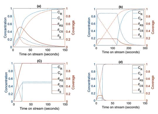
**Figure 5.** Estimated reactant and product concentration profiles (**left** *y***-axis**) and surface species coverages (**right** *y***-axis**) with respect to time: sensitivity analysis for Mechanism I, (**a**) with reduced  $k_1$  by 100% and increased  $k_{-1}$  by 10% (**b**) increased  $k_2$  by 10% (**c**)  $k_C = 0.36$  (**d**)  $\tau = 5$  s.
