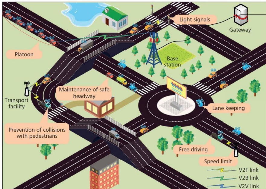
Figure 2. A representation of connected vehicles and infrastructure [18].
