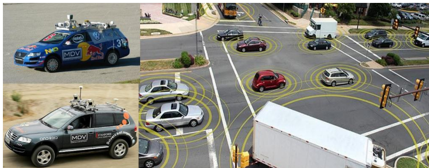
Figure 1 A graphical depiction of connected autonomous vehicles equipped with technologies such as Lidar, video camera, positioning estimator, distance sensors. These vehicles can “talk” to each other exchanging information such as vehicle size, position, speed, heading and turn signal status. (Image extracted from www.trucks.com and adapted).
