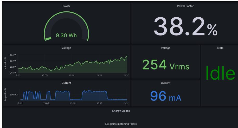
Fig. 5: Energy-related data monitoring and visualisation dashboard for shop-floor engineers and maintenance technicians.
