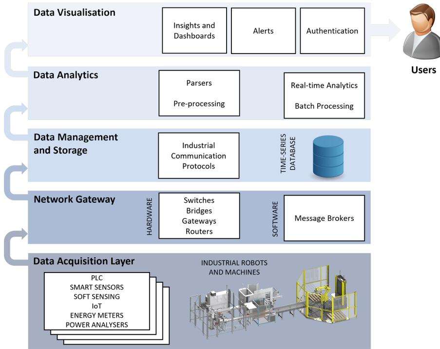
Fig. 1: The proposed architecture for industrial robotic assembly.
