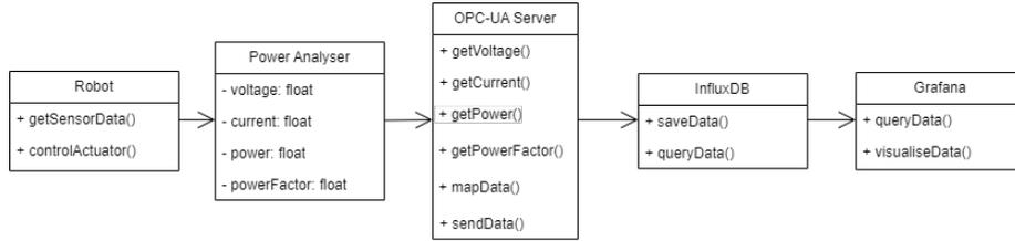
Fig. 4: High level system information flow.
