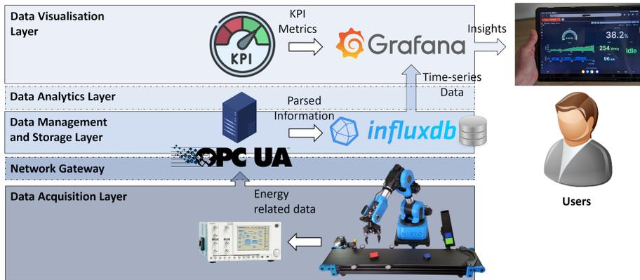
Fig. 2: Energy-related information flow and implemented technologies (Layers that are outlined with a dashed line are not considered within the scope of this study.).
