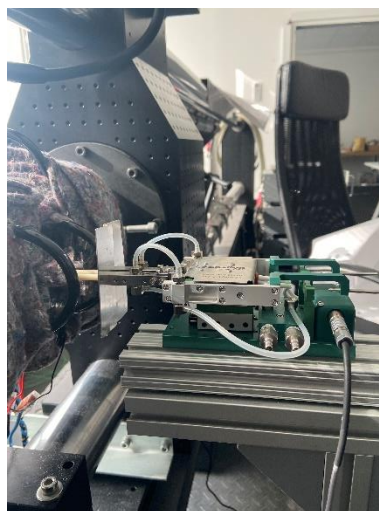
Figure 5.7: The extensometer placed on the grips of the compression rig.
