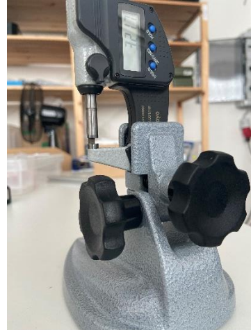
Figure 5.3: a) Micrometre used for measuring samples dimensions b) Sample placed on the micrometre.
