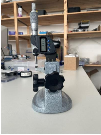
Figure 5.3: a) Micrometre used for measuring samples dimensions b) Sample placed on the micrometre.
