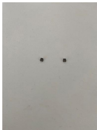
Figure 5.2: The SMA samples used for DSC testing and the mechanical loading.
