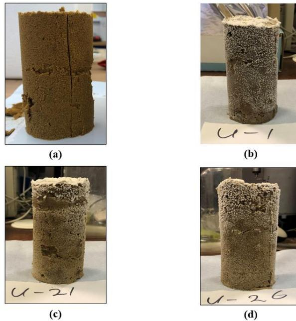
**Figure 4:** Biocemented images of soil (a) Biocementation using water only (b) U-1 CA-producing bacteria (c) U-21 (d) U-26 CA-producing bacteria.
