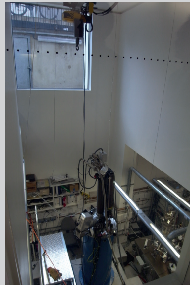
▲ Figure 3.7 The London Centre for Nanotechnology: double height basement laboratory - with subsurface daylight window and built-in crane - for single atom
