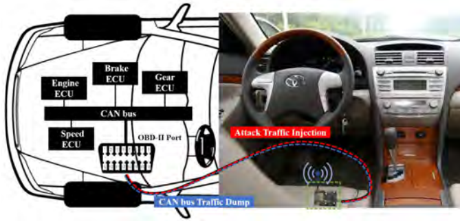
Fig. 2. Components of prototype system designed to evaluate Aiden. The system can inject attacks through the OBD-II interface. The injection process can be done in either of two communication modes: wired or wireless.
