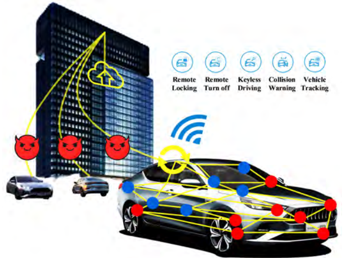
Fig. 1. An attack enters into the CAN bus of a modern/autonomous vehicle through wireless channels, and the in-vehicle ECUs connected by the CAN bus are compromised. Because of the intrinsic associations among different ECUs to take actions, the attack from the compromised ECUs easily causes cascading failure to make the vehicle deviate from a safe operational regime.
