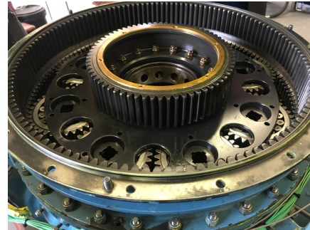
Figure 2. Demonstration of 2 nd planetary sun gear and ring gear
