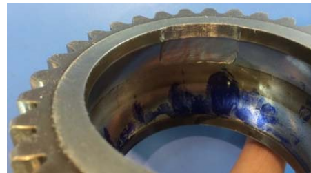
Figure 3. Major defect seeded at planetary bearing outer race
