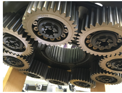
Figure 1. Demonstration of 2 nd planetary gear/ bearing set
