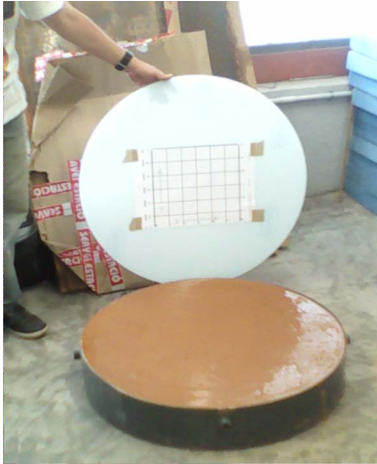
Figure 3 – Specimen and PMMA plate with grid to guide the device
