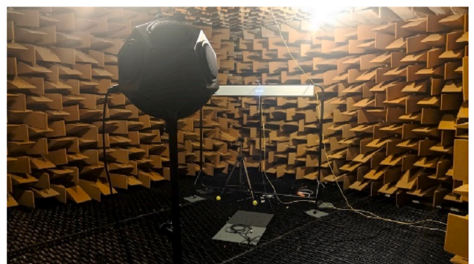
Fig. 1. Test Microphones with Pink Noise using Substitution.
