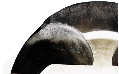
(b) Melted section of valve pockets
