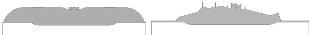
Figure 5.19: Section views of combustion chamber. Left: plane passing through both cylinder and crank-shaft axes. Right: perpendicular to the first plane, passing through squish land.
