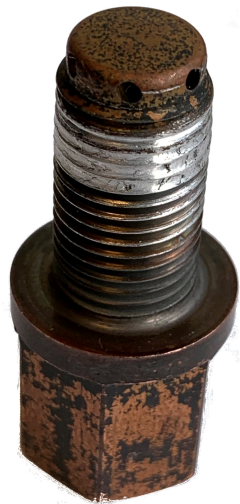
(a) Post test pre-chamber part with melted aluminium on threads.
