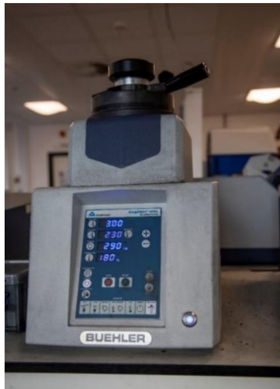
Figure 4.7 - Buehler SimpliMet 4000 used to mount all samples at material's lab at Warwick University.
