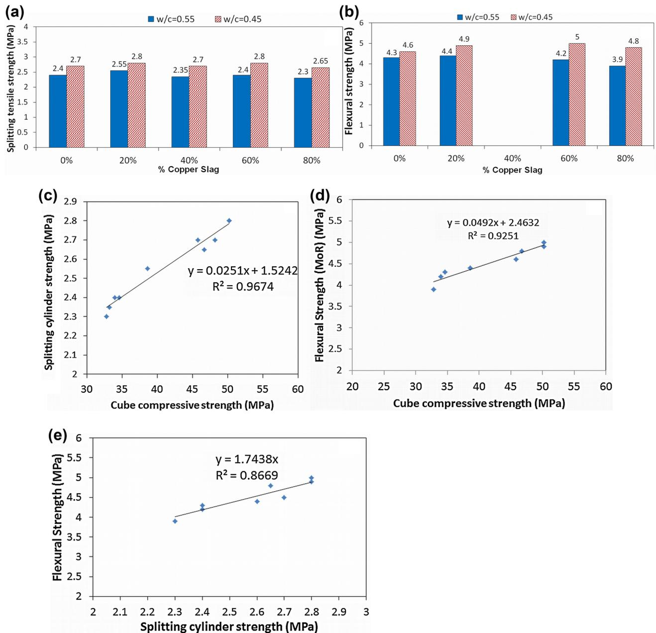
**Fig. 4** Indirect tensile strength tests: **a** splitting tensile strength; **b** flexural strength; **c** correlation of splitting cylinder strength with cube compressive strength; **d** correlation of flexural strength with cube
