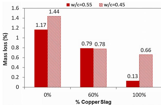
**Fig. 7** Accelerated corrosion testing results
