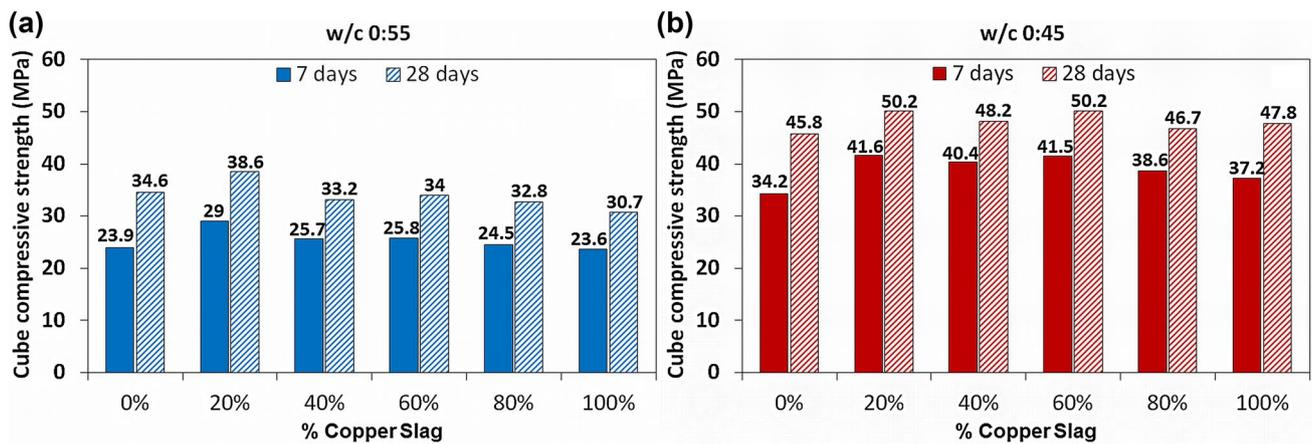
**Fig. 3** 7 and 28-days curing compressive strengths of mixes: **a** w/c=0.55; **b** w/c=0.45
