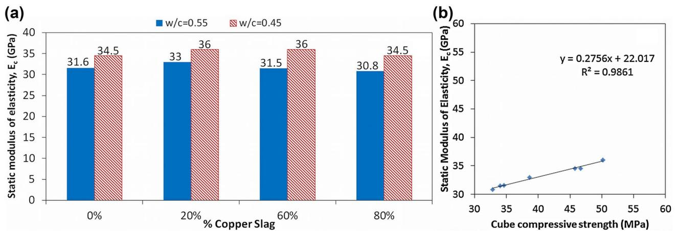
**Fig. 5** Static modulus of elasticity tests: **a** Static modulus of elasticity values; **b** correlation of static modulus of elasticity with cube compressive strength
