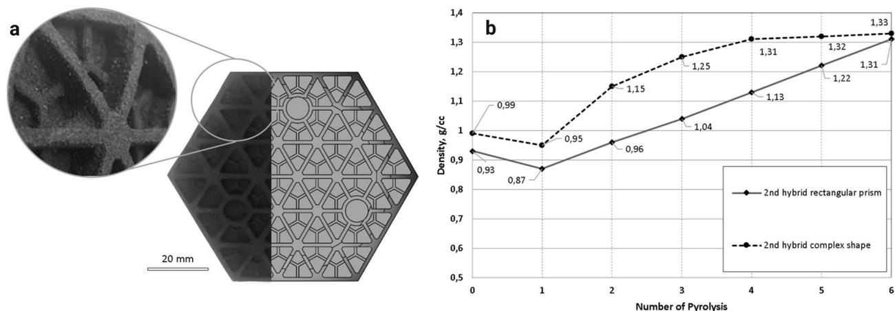
**Figure 9.** (a) Overview of graphite BJP complex structures densified through PRBI and pyrolysis cycles; (b) dependence of the hybrid complex-shape sample's density on the number of pyrolysis. The 2nd up to 6th pyrolysis was applied after PRBI.
