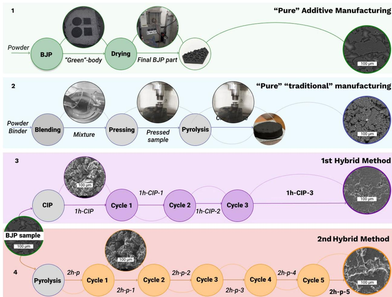
**Figure 2.** Process flow showing production of graphite using different production routes where *BJP* Binder Jetting Printing, *CM* compacted moulding, *CIP* Cold Isostatic Pressing, Cycle is the sequence of Impregnation—Drying—Pyrolysis.
