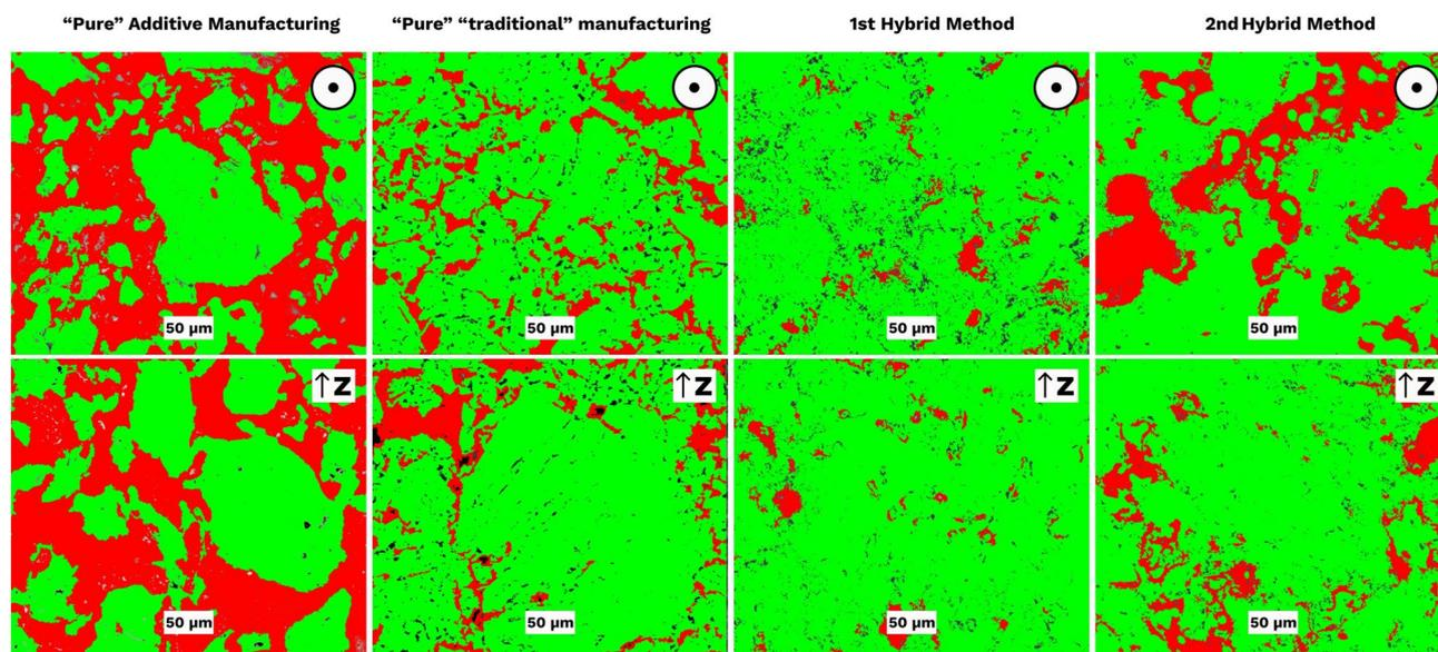
**Figure 4.** Image analysis of optical microscopy images of crosscuts in XY- and Z-planes. The black arrow points at the build/pressing direction (Z), i.e., perpendicular to the layers; the black circle with the point in the center corresponds to XY plane—parallel to layers.
