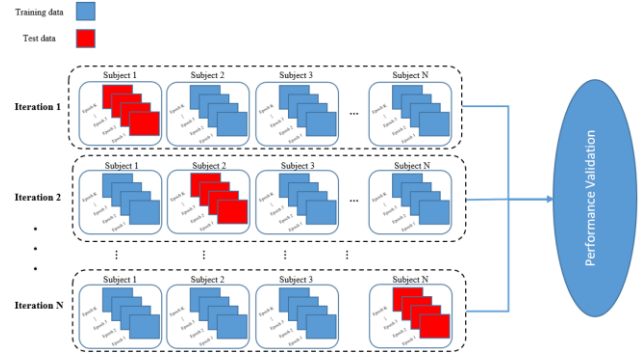
Figure 5. Representation of the LOSO-CV method. In each iteration, a classifier is trained using a training set (blue) and then tested using the test set (red) to obtain the necessary accuracy. The number of iteration is equal to the number of subjects.
