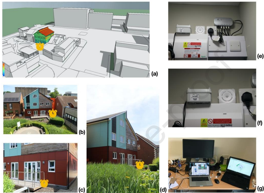
Fig. 13. (a) 3D rendering model of archetype house and surrounding built environment. (b) The location of weather station installed in the Innovation Park site. (c) The weather station was installed beneath the decking space. (d) The position of weather station installed in the property. (e) The location of environmental monitoring device mounted on the wall in the battery room. (f) The main environmental recording station. (g) The environmental recordings were monitored and data extracted for experimental analysis by using highly efficient custom-made computers provided by the author.
