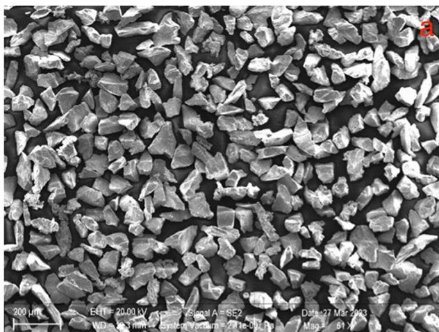
Fig. 1. (a) Titanium powder (Metco 4012A) observed through a scanning electron microscope for understanding the morphology and, (b) the size range
