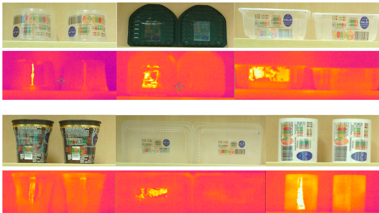
Figure 4. An example of a set of plastic objects with standard labels and labels coated with the IR-reflecting oxide films. The objects on the right are fitted with uncoated labels, while the objects to the left are fitted with a coated label.
