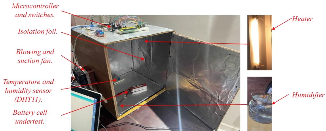
**Figure 3-2** Climatic chamber to control temperature and humidity.
