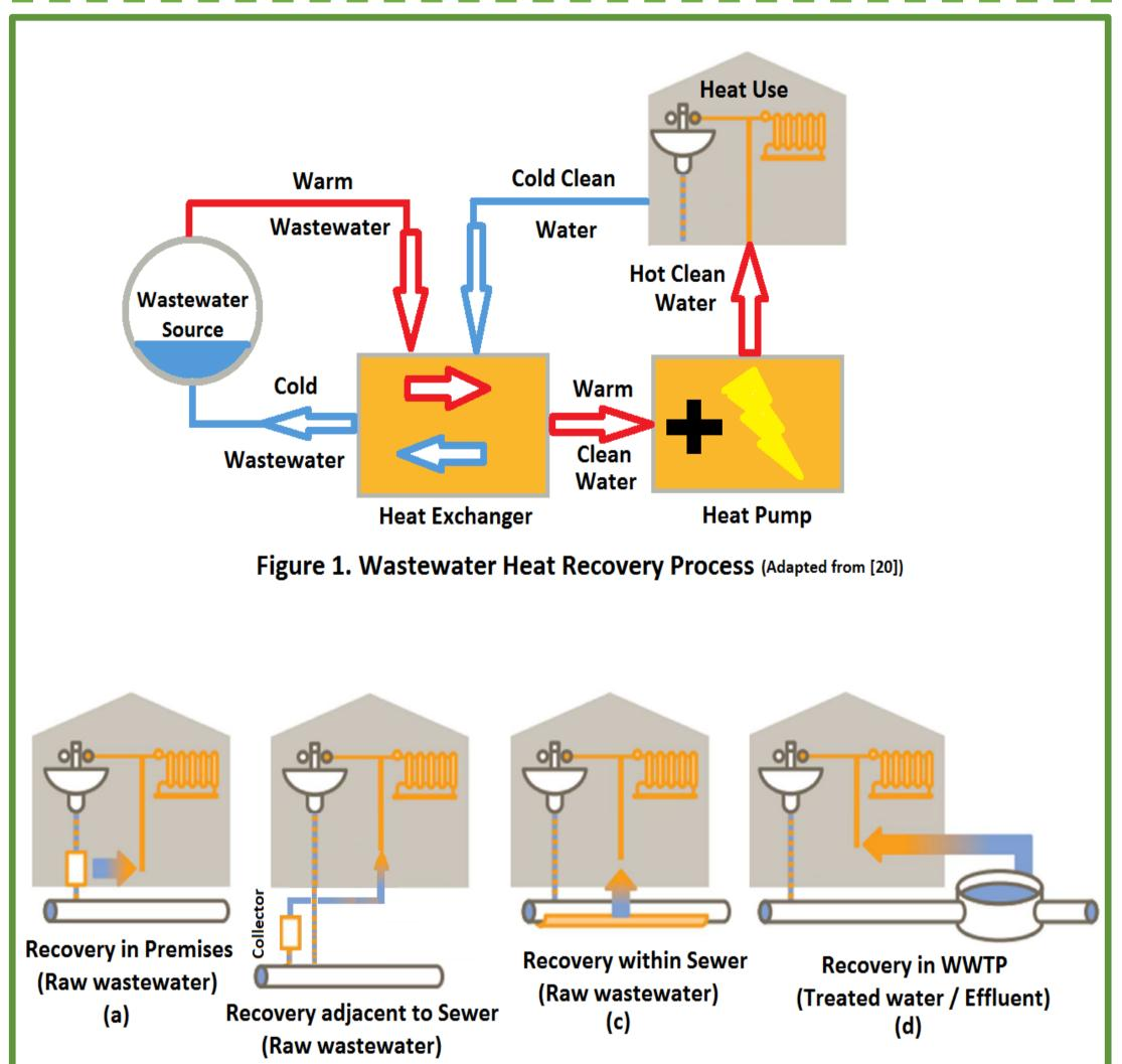
Figure 2. Possible Heat Recovery Locations (Adapted from [21])
