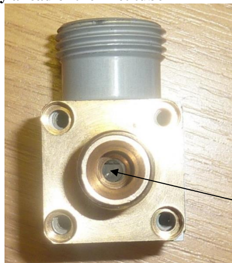
Figure 6-14 Side view of GA3030 aluminium body and brass inlet showing the flat impingement site directly ahead of the inlet tube
