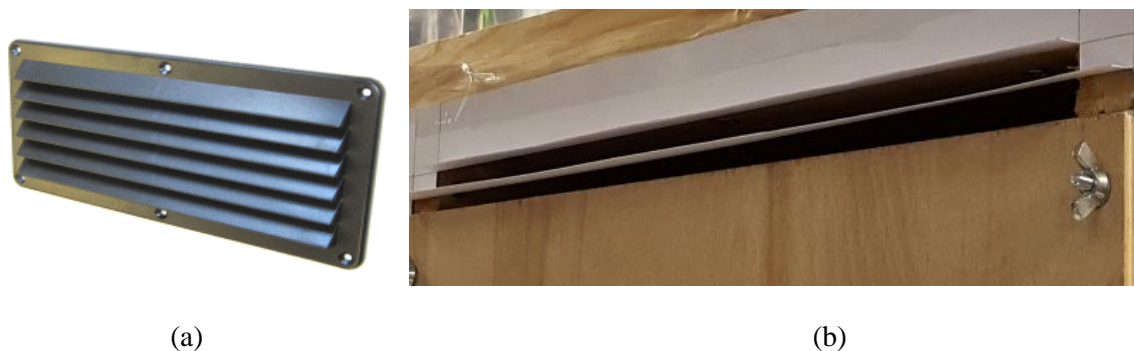
Figure 1 (a) Standard louvre vent (b) Fuel cell enclosure rig, louvre ventilation opening design
