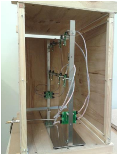
(c) Frame sensors in enclosure
