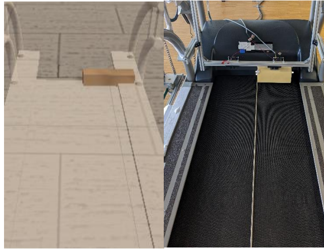
Figure 21: Obstacle setup for virtual and physical environments. In the physical environment, a foam obstacle with the same dimensions as those in the virtual environment was attached to an electromagnet which released the obstacle at foot touchdown of the crossing leg.
