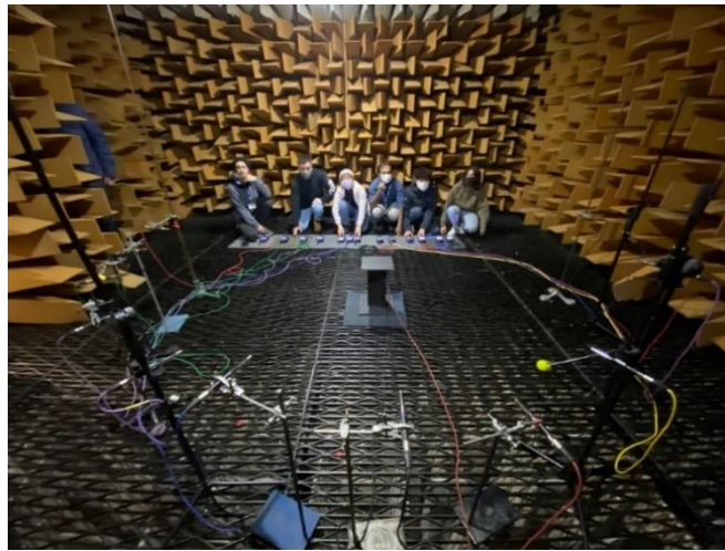
Figure 9 - Speech directivity measured at 15o intervals in an anechoic chamber. Averaged speech directivity (dBA) is given in figure 10 based on 4 native English talkers
