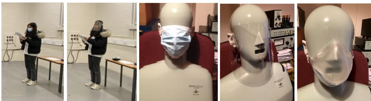
Figure 1- Native speaker and HATS wearing Surgical, Visor and Prototype Mask
