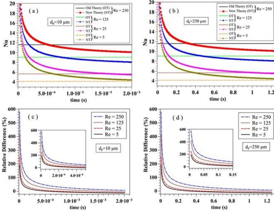
Figure 3. Transient Nusselt correlation compared with steady-state Ranz-Marshall correlation at different Reynolds numbers and diameters, Dbouk and Drikakis (2020) [20]
